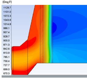
CFD Model of Flue Gas Temperature
